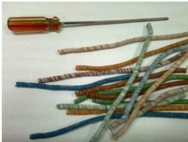
Cut it to make coils between 5 to 10mm, or three wind each. Make enough coils to fill 8 cm diameter 5cm height. Correct direction of winding is very important. Must be like this:
