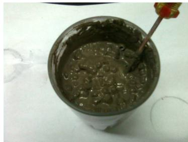
Pour it into the mould. You can also put the coils first, then pour. Mould must be a cylinder. 8cm diameter 5cm height is for outdoor use. Use 7cm diameter for indoor or vehicle. :
