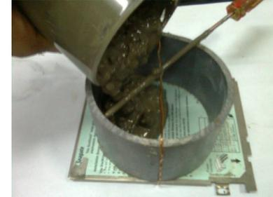
Make sure the coils are packed, no cement without coils, remove excess cement.
