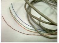
Remove the outer insulation and undo the twist. Then roll/wound it on a 3mm rod. The direction of winding must be clock wise if seen going further away from you:
