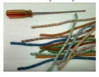
Cut it to make coils between 5 to 10mm, or three wind each. Make enough coils to fill 8 cm diameter 5cm height. Correct direction of winding is very important. Must be like this:
